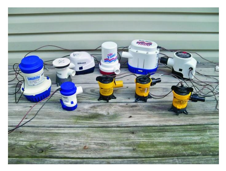
The low-capacity bilge pumps we tested included 10 models from Shurflo, Johnson Pumps, Rule/ITT, and Attwood.
