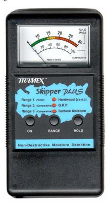
If an osmosis prevention or treatment is to be carried out, readings must be lower than 14% H<sub>2</sub>O (i.e. 'in the green') before any epoxy materials are applied. The same readings are required when applying polyurethane finishes to topsides and superstructures, or when carrying out laminate repairs.
